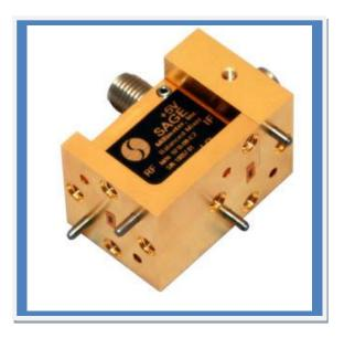
**Model SFB-06-E2** is a D-Band, externally biased balanced mixer. The mixer employs high performance GaAs Schottky beamlead diodes, balanced configuration and proprietary bias circuitry to produce superior RF performance with very low LO pumping level. The low LO pumping level is desirable feature at higher millimeterwave bands.
